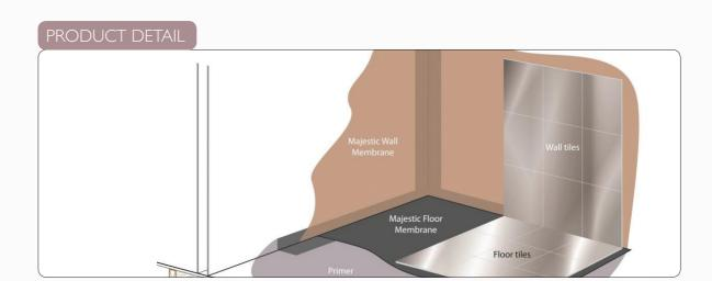
Majestic Wall Membrane is a flexible coating for waterproofing wall surfaces prior to the application of ceramic tiles and natural stone in wetroom and other critical areas.
