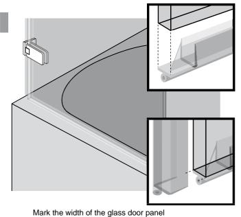
on the 1915 under-door seal (2); cut the seal to length. Prepare the seal as shown to allow it to intersect with the 1936 door-to-glass seal and slide it onto the bottom of the door.
