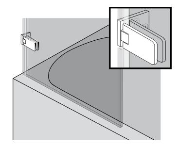
The 1929 door-to-wall seal (1) should be cut into three pieces and fit vertically above, between and below the hinges. You must notch the seal to sit inside the hinge as shown below. on the end of the bath screen. Note: the seal should extend down below the bottom of the door to touch the lip of the bath. Slide the sections into place on the door.
