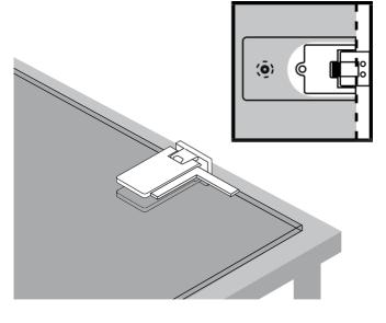
Disassemble the hinges, being careful not to damage the polished surfaces. Place the hinges and faceplates either side of the hinge slots in the glass bath screen, with gaskets inserted and wall screw plates facing inwards; loosely screw the hinges and faceplates together.
