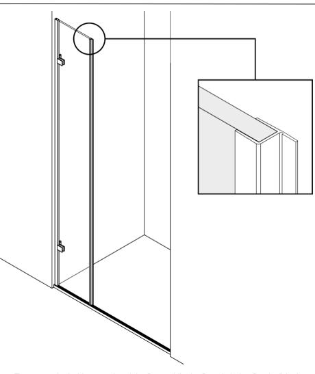
To protect the In-Line panel and the Door while the Door is being fitted, slide the vertical seal on to the edge of the In Line panel. Push it down to touch the underframe and trim it level with the panel at the top.
