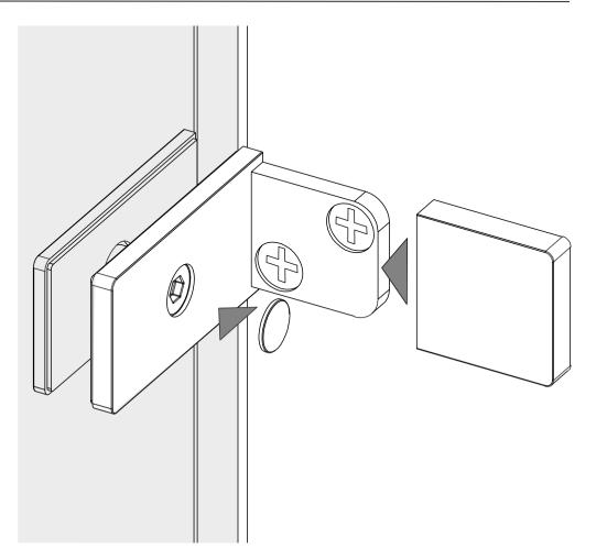
ensuring the black plastic washers are located in the holes on both sides of the glass.
