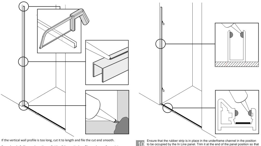
Run a bead of silicone along the wall side of the vertical profile, as shown. Screw it in place.
