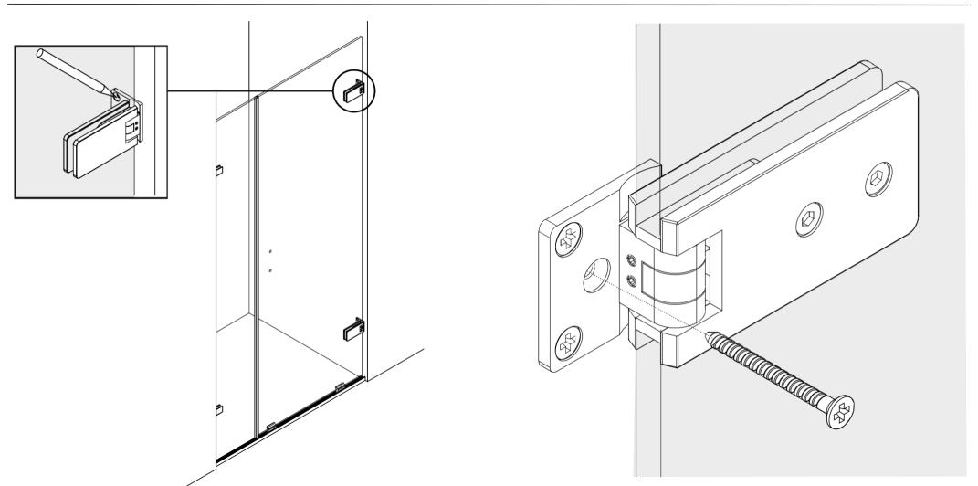
Ensure that the Door is in the correct position, aligned with the In Line panel and plumb vertical. Mark the 6 hinge screw holes on the wall and then remove the Door, drill 7 mm holes and insert the wall plugs provided.
