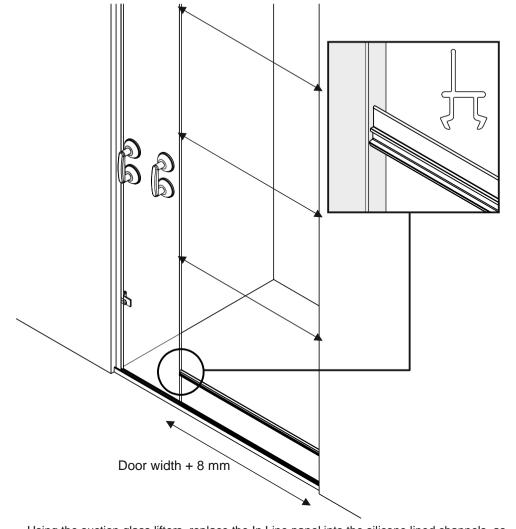
Using the suction glass lifters, replace the In Line panel into the silicone lined channels, as marked on the underframe. Make sure that the gap for the door is correct and that the clear plastic Underframe Insert fits snugly between the In Line panel and the wall over the full height of the door aperture.
