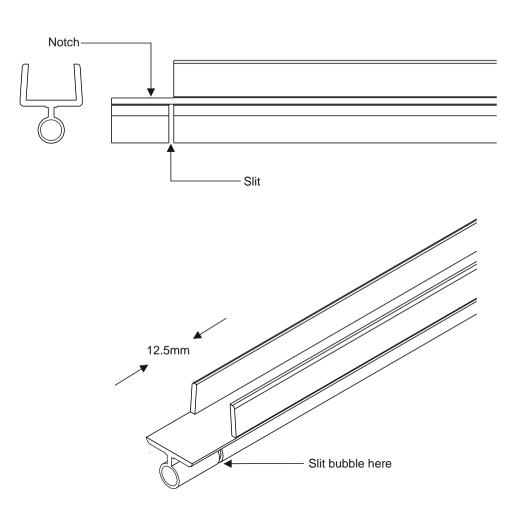
The other length of vertical seal is to be cut in 3 sections to fit to the door above, below and between the hinges.
