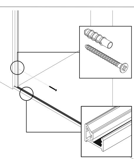
Drill 4.5 mm holes where marked and insert wall plugs. Reposition the vertical profile and insert the top and bottom screws to hold it temporarily in place.
