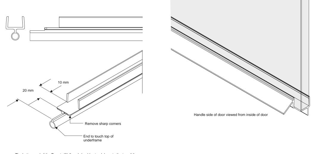
The bottom end of the Door to Wall seal should extend down to the top of the underframe but should be notched as shown so that it does not interfere with the horizontal seal which will be fitted to the bottom of the Door.
