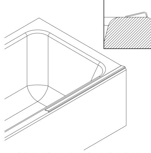
Position the underframe on a substantially flat section of the rim of the bath approximately as shown, with the gentle ramp facing inwards and one end touching the wall.
