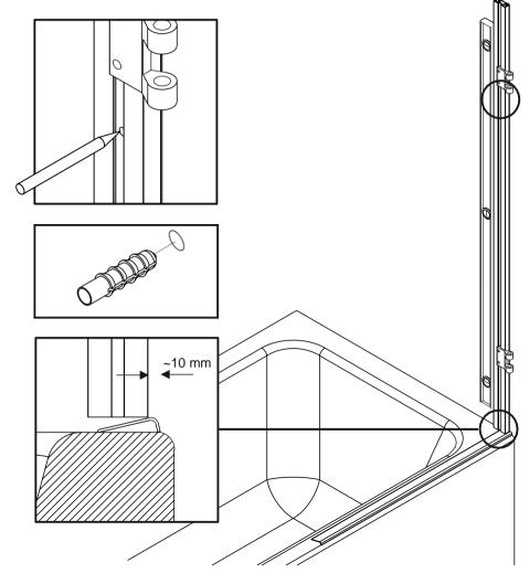
Position the vertical wall profiles so that their bottom corner rests on the underframe, about 10 mm inboard of its edge as shown above.
