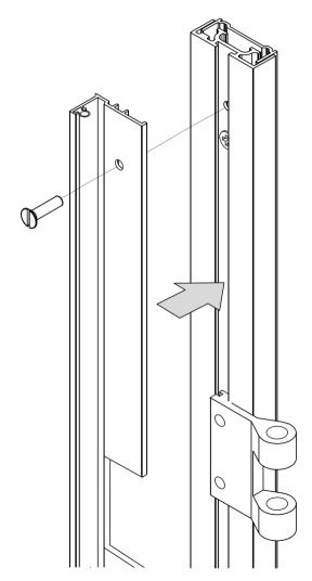
Once you are satisfied that the face of the wall profile is at 90 degrees to the rim of the bath, fully tighten the wall screws and replace the cover plate as shown.
