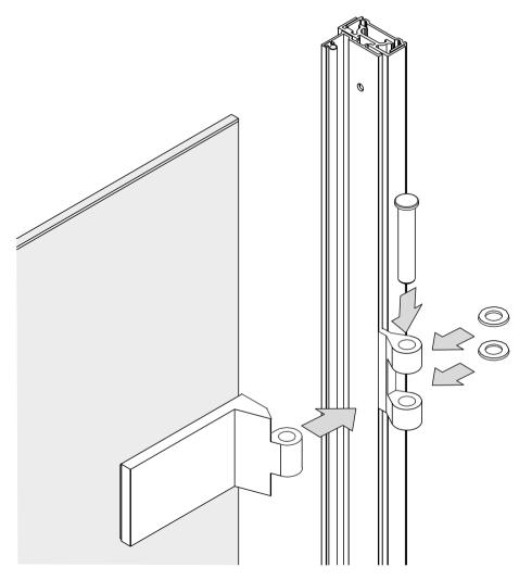
Offer up the assembled glass leaf. Place the plastic washers in between the moving parts of the hinge as shown and drop the retaining pins into place from above.
