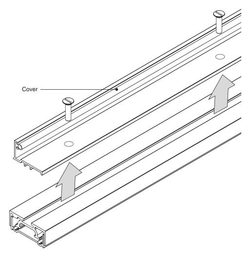
Unscrew and separate the cover from the wall profile assembly as shown .
