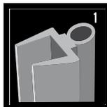
The other 1929 door-to-wall seal should be cut to fit on the exposed vertical edge of the glass door.
