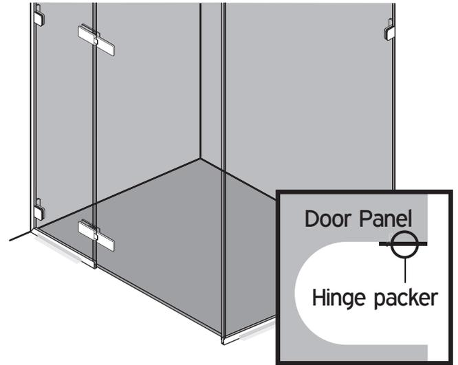
**29** Position the hinges on the fixed panel centrally in their slots and use a set square to ensure they are square to the edge of the glass; the gaskets should be neat and flush, and the end of the glass door should not protrude beyond the hinges. Tighten the Allen bolts.
